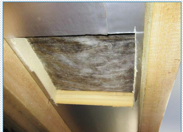
Picture 2: Sampling of the test specimen
